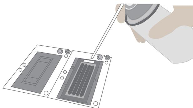
Figure 40 Cleaning the Flow Cell
