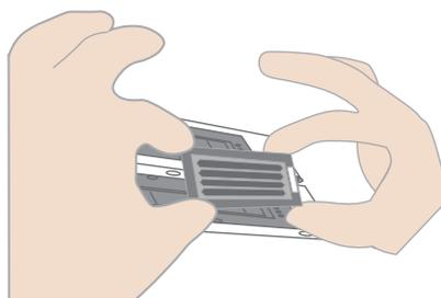
Figure 39 Loading the Flow Cell
