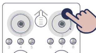
Figure 10 Seal the loading wells tightly of FCL SE50/FCL SE100 /FCS SE100 cartridge
