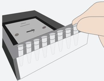
DNB loading: load the DNB into sequencing Flow Cell.
