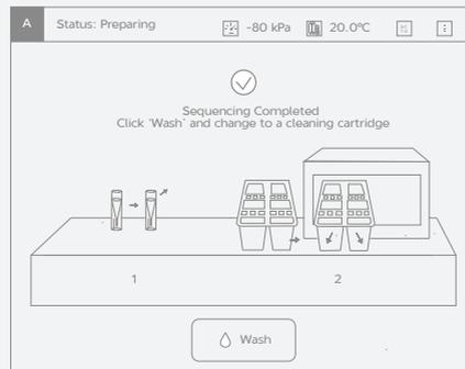
Device maintenance: perform device maintenance when sequencing is completed.
