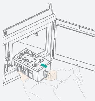
Loading the reagent cartridge into the sequencer.
