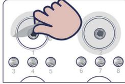
Figure 17 Removing the seal from FCL PE100/FCL PE150/FCL PE200/FCS PE100/FCS PE150/FCS PE300 cartridge after mixing
