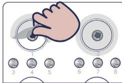
Figure 12 Removing the seal from FCL SE50/FCL SE100 /FCS SE100 cartridge after mixing
