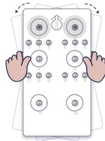
Figure 21 Mixing reagents after loading
