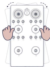
**Figure 16** Mixing reagents after loading
