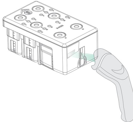
Figure 34 Reagent cartridge information entry interface
