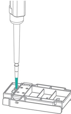
Figure 6 Loading samples using MGIDL-200H
