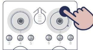
Figure 20 Sealing the loading wells of FCL sRNA SE50 cartridge
