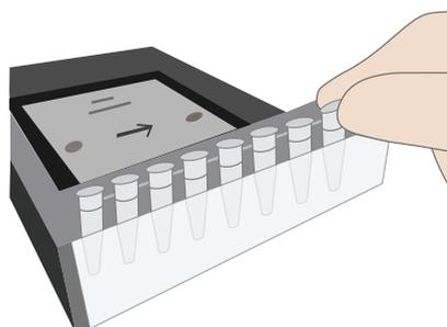
Figure 5 Placing the loading samples
