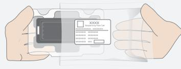
Preparing a new Flow Cell: take out the Flow Cell from package and inspect to ensure the Flow Cell is intact.
