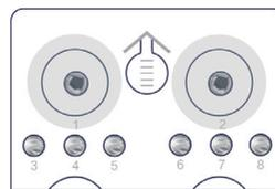
**Figure 14 Sealing the loading wells of FCL FCL PE100/FCL PE150/FCL PE200/FCS PE100/FCS PE150/FCS PE300 cartridge**
