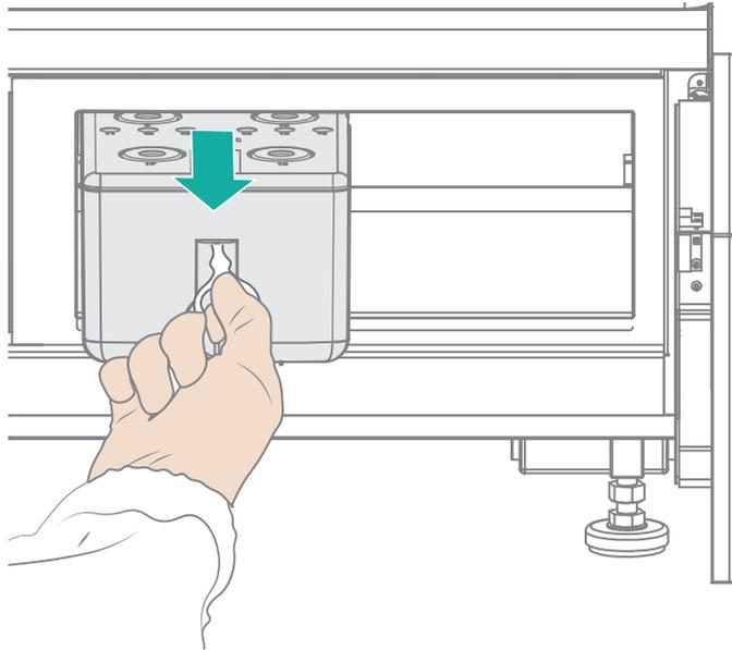
Figure 35 Removing cleaning cartridge
