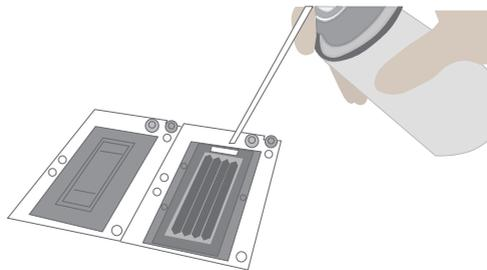
Figure 38 Cleaning the Flow Cell stage
