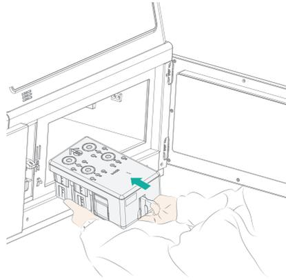
Figure 37 Sliding the new reagent cartridge into the reagent compartment
