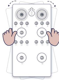
Figure 11 Mixing reagents after loading
