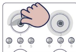
Figure 22 Removing the seal from cartridge after mixing
