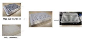
Note: the usage of Adapter+96-well half skirt PCR plates is shown in the upper figure (Adapter reusable), and it can directly replace the Hard-shell thin-well skirted PCR plates, white shell/clear well (MGI, 1000012059).
