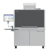
MGISTP-7000 a high-throughput automated sample transfer processing system. It integrates tube decapping, tube recapping, barcode identification, automated liquid transfer and negative pressure protection. It decreases steps and delivers the quality and reliability you expect. You can transfer 192 samples from screw cap transport tubes or plain tubes to 96-Well Microplates in 40 minutes.
