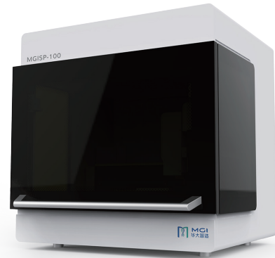
Figure 2. DNA Sequencing Library Preparation System MGISP-100
