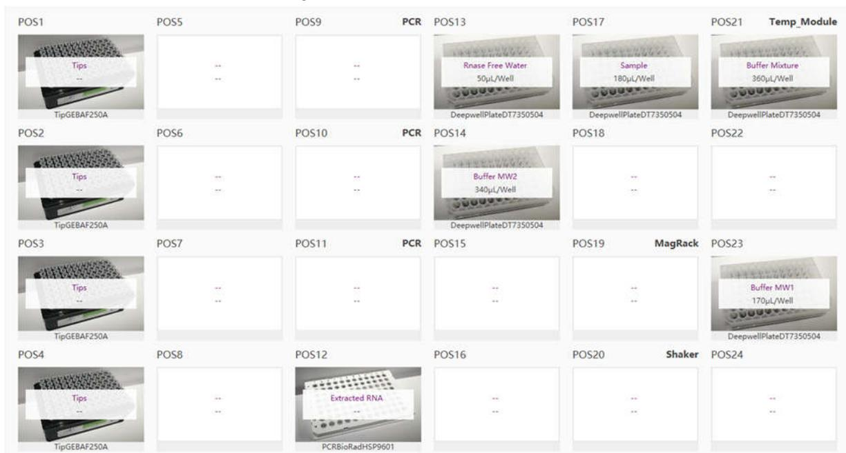
Figure D-6 First Phase Operation Deck Arrangement
