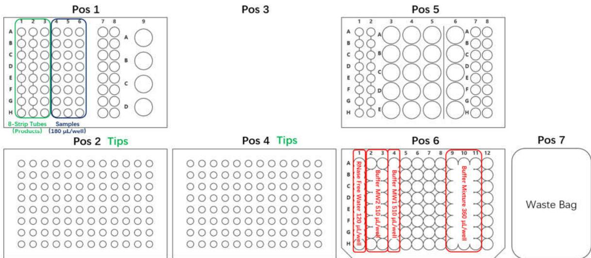
Figure E-12 Operation deck layout for 24 rxn
