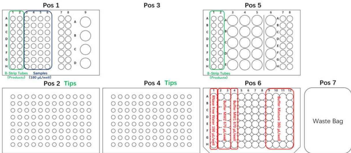
Figure E-13 Operation deck layout for 32 rxn
