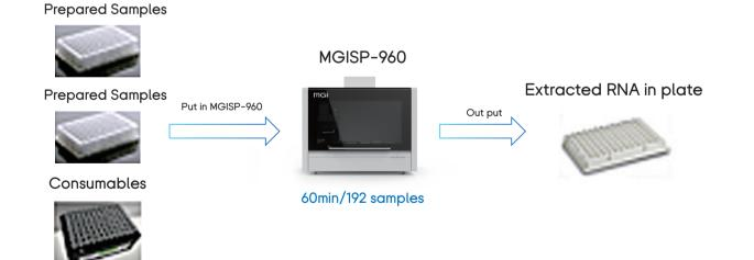
The above introduction is based on 96 samples / run as an example. The operation mode of 192 samples / run is quite similar and required only the selection of the corresponding script in the software.
