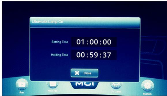
Figure 17 UV lamp setting interface
