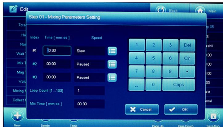
Figure 12 Mixing parameter setting interface
