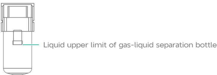
**Figure 14** Upper limit of the liquid level of the gas-liquid separation bottle
