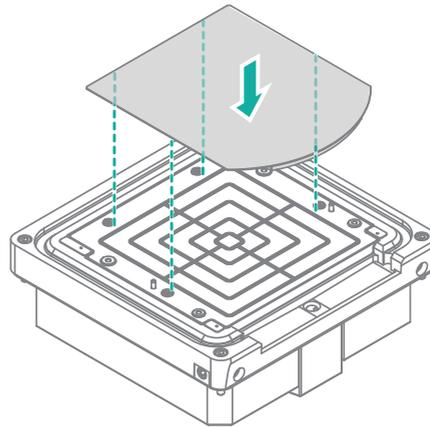
Figure 15 Placing a slide
