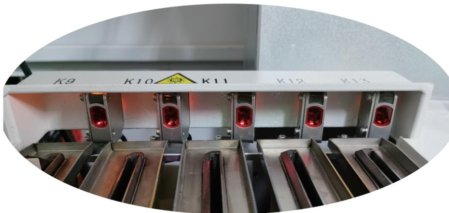
Figure 18 Photoelectric sensor
