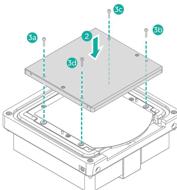
Figure 17 Installing the glass cover plate
