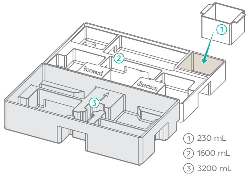
Figure 26 Washing container (0.1 M NaOH)
