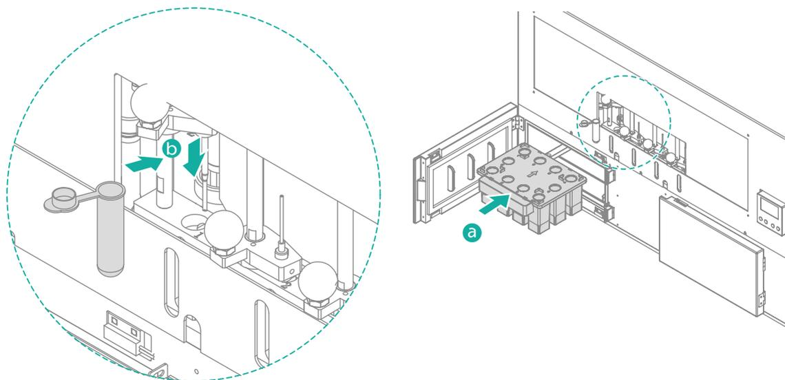
Figure 13 Loading DNB washing centrifuge tubes and pure water washing cartridge
