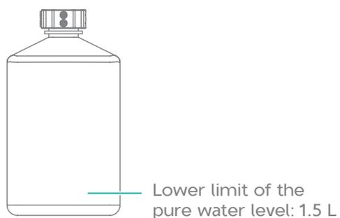
Figure 11 Lower limit of pure water level
