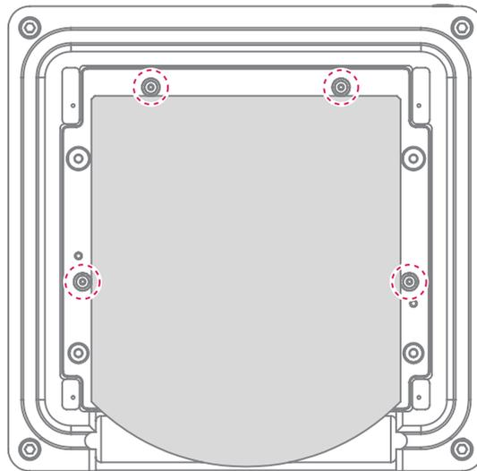
Figure 16 Aligning the slide with positioning posts
