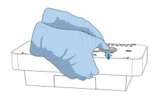
5. Hold the A and B sides of the cartridge with both hands by following the marks A and B on the cartridge, and invert the cartridge for 10 to 20 times to mix the reagents thoroughly. Pierce the MDA well with a clean 1 mL pipette tip. Then, gently tap the cartridge against the desktop to remove bubbles.
