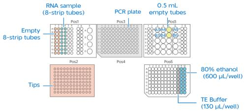
4. Add the reagents to wells of Pos 5 according to the table below:
