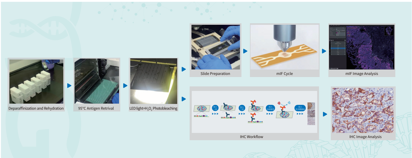
Figure 2. The schematic diagram of the workflow for tissue section samples under mIF or IHC staining. The entire process can be summarized as follows: (1) in the fume hood: deparaffinization, hydration, antigen repair, and quenching; (2) mIF workflow: preparation before loading to DNBSEQ-G400RS FluoXpert, imaging, and data analysis; (3) IHC workflow: IHC staining, image stitching and image analysis under a microscope.
